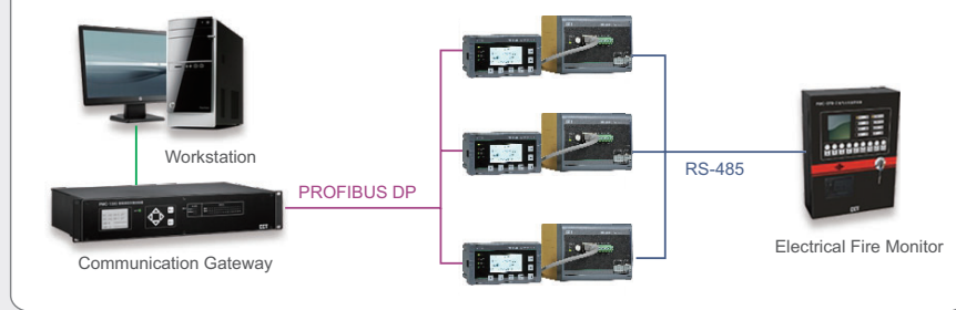
PMC-550A's Connection Diagram for Electrical Fire Monitoring
