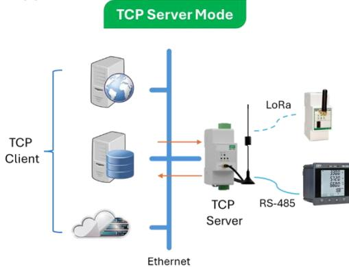
In TCP Server mode, the TCP Clients can initiate and establish the connection. The TCP Server shall listen to the specified Local IP Port and wait for the TCP client to connect. The data sent by the downstream RS-485-enabled or Lora devices will be transparently transmitted to all successfully connected TCP clients by the TCP server.
