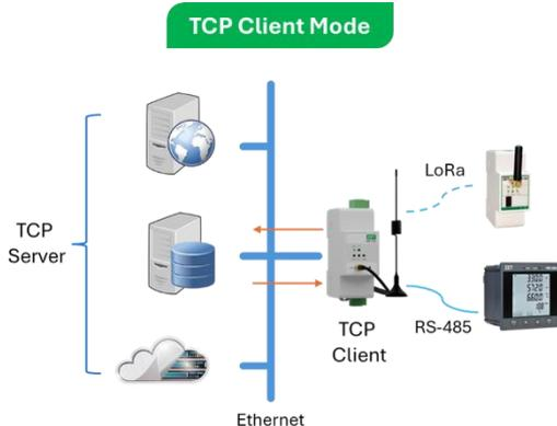
In TCP Client mode, the TCP Client initiates a TCP connection to the target IP address and port. If the connection fails, the TCP client will try to reconnect after the Reconnect Interval, until it succeeds. Afterwards, the RS-485-enabled or LoRa devices communicate bi-directionally with the TCP server through the TCP client.
